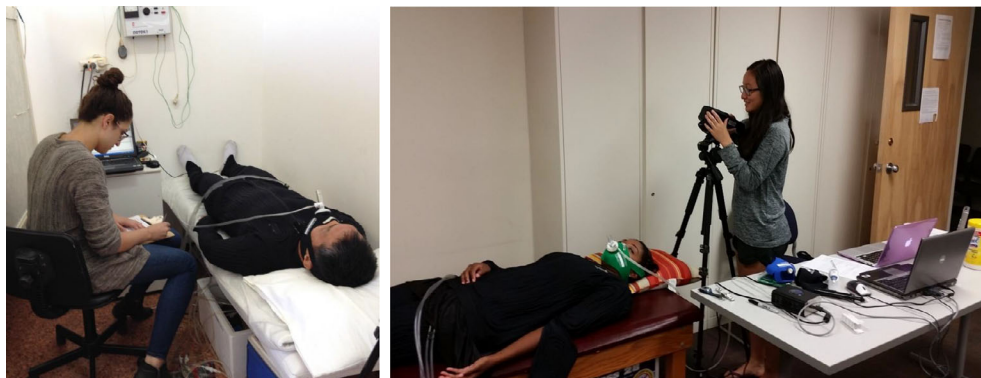
FIGURE 1 Examples of water-perfused suit, water pump, indirect calorimetry and thermal imaging set-up
